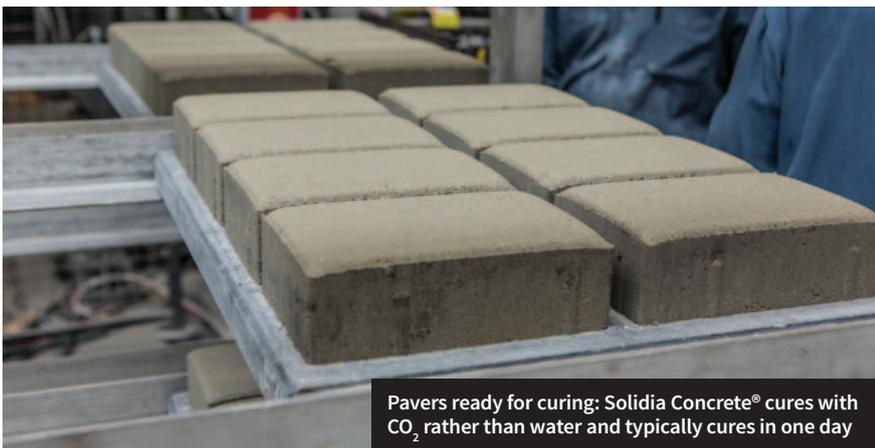
Pavers ready for curing: Solidia Concrete® cures with CO<sub>2</sub> rather than water and typically cures in one day
