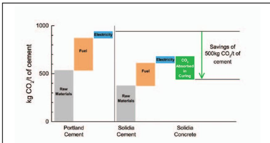
Figure 1: comparative CO<sub>2</sub> emission from raw material, fuel and electricity for Portland cement (~940kg/t) and Solidia Cement (660kg/t). The curing reaction in Solidia Cement consumes CO<sub>2</sub> (~240kg/t) resulting in up to 500kg/t reduction in CO<sub>2</sub> emission
