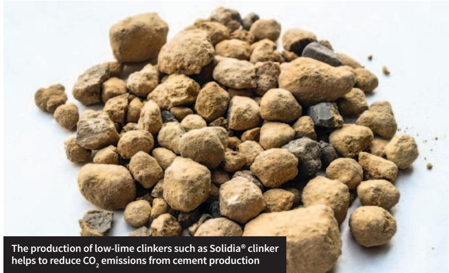
The production of low-lime clinkers such as Solidia® clinker helps to reduce CO<sub>2</sub> emissions from cement production
