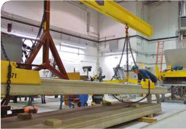
Figure 3. Solidia Concrete hollow core slab being removed from the extrusion bed after a 24 hour CO 2 -cure.
