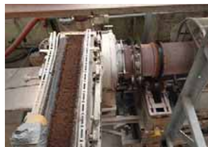
Figure 1: Raw meal fed into the 0.3m inner-diameter, 7.6m-long rotary kiln at IBU-tec.
