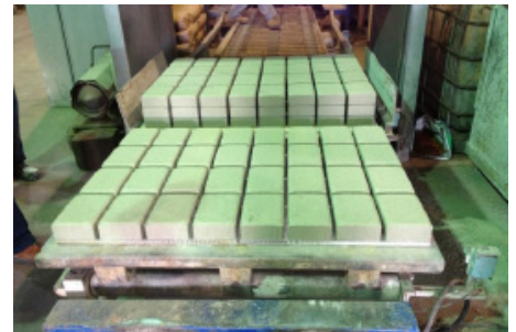
SOLIDIA CONCRETE PAVERS READY FOR CO 2 CURING
