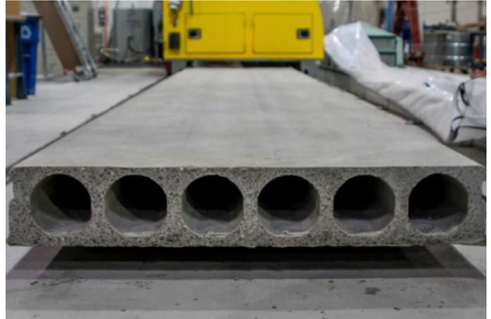
**SOLIDIA CONCRETE™ HOLLOW CORE OFFERS ENERGY AND RESOURCE EFFICIENCIES**
